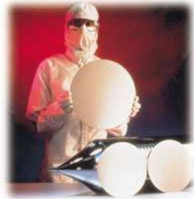
*Taisil Electronic Materials Corporation's silicon wafer and crystal ingots*
