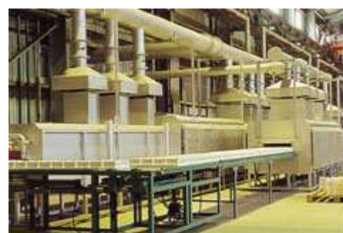
Production line of sinter disc bodies for PTCR degaussers
