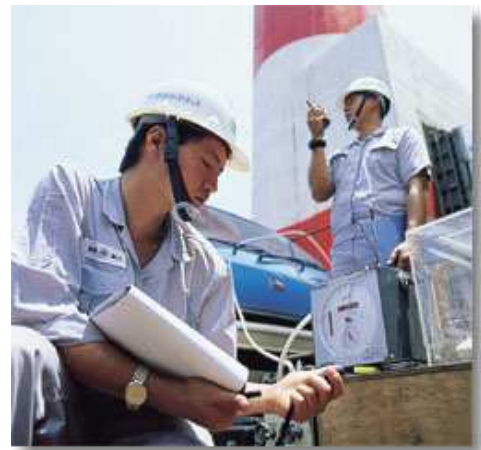
Testing for particulate emission at a gas duct
