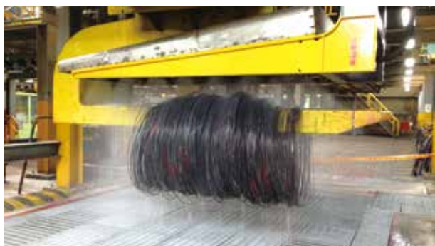
Sprinkling special lubricants to reduce the friction coefficients among coils
