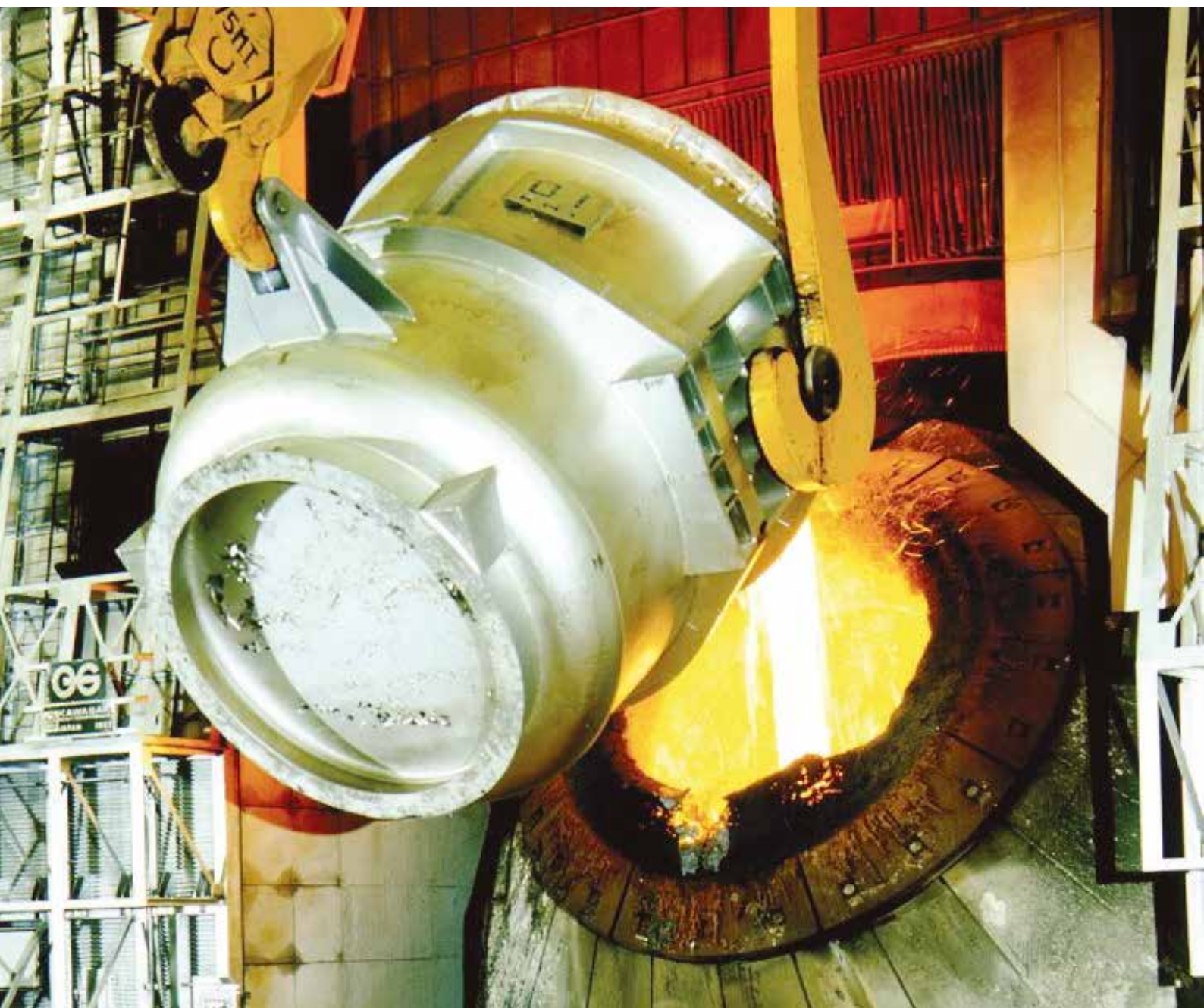
Pouring of molten iron into the BOF
