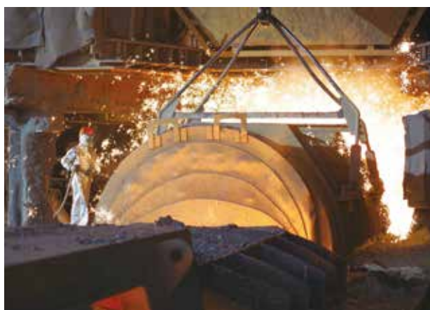
Tapping of iron at a blast furnace
