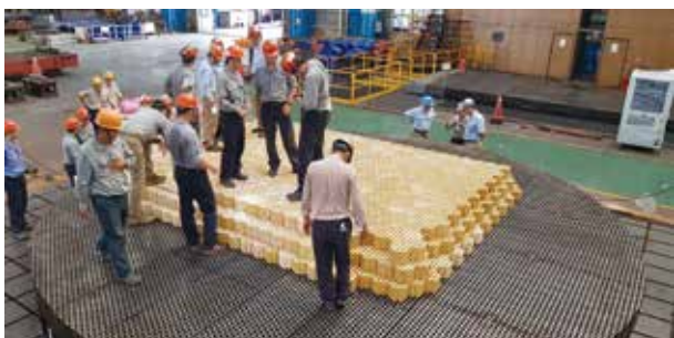
Independent development of checker brick support bases for hot-blast stoves
