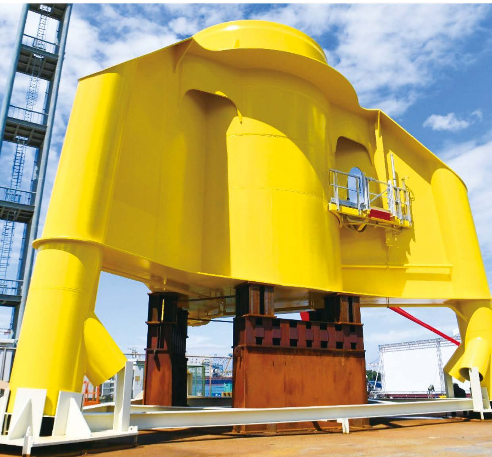
Taiwan's first transition piece mock-up to a jacket foundation
