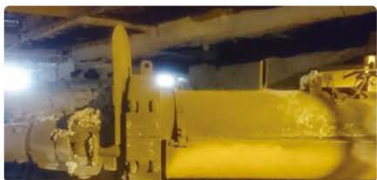
A mud gun machine at a blast furnace tap hole
