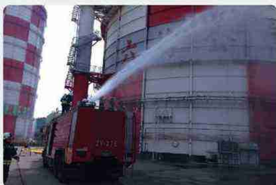
Cooling of the temperature by spraying water from fire engines
