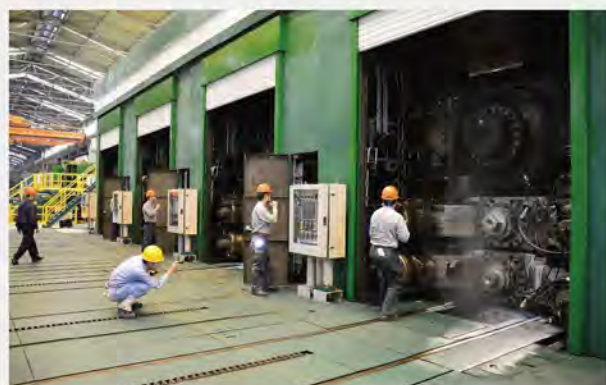
Test runs of the hot strip finishing mill
