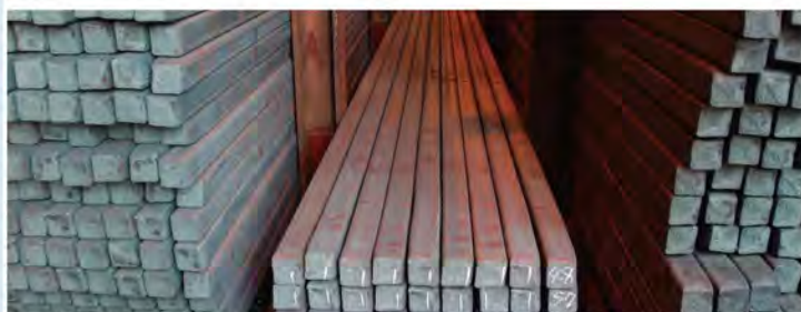
Storage yard of billets
