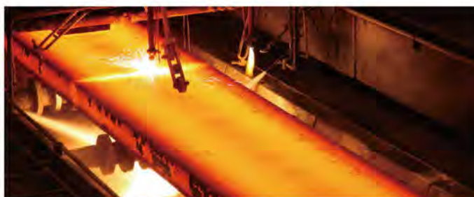
Flame cutting on slabs
