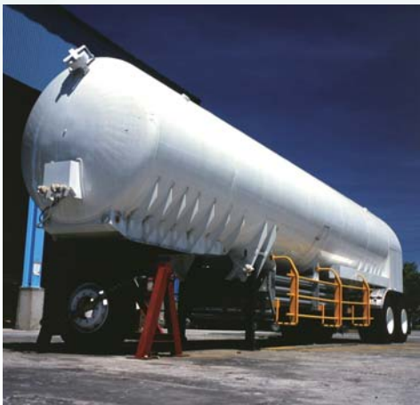
Tank truck was made of pressure vessel steel.
