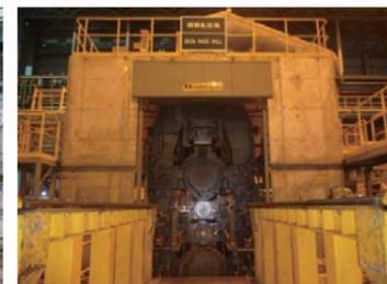
After the annealing, the strip is slightly rolled by the skin-pass mill to avoid the common defect called stretcher strain and adjusting mechanical properties. The strip surface roughness is also determined by this stage.
