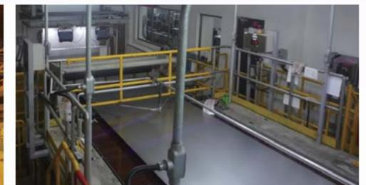
The entire coil strip thickness, width and surface quality are checked by automatic inspection system and well-trained inspectors in this stage. After the oil applied over strip surface, the product coil is cut into specified mass.
