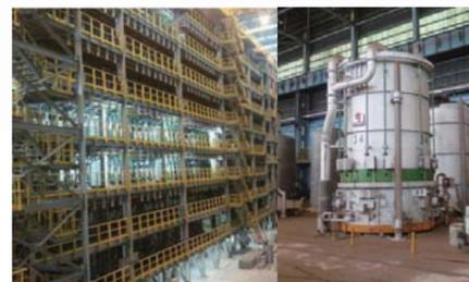
The steel strip is significantly hard and brittle after cold rolling which the grains are elongated along with lots strain energy. To obtain the desired mechanical properties of strip, the coils shall be piled and covered by the box which called batch annealing or the strip is continuous treated in furnace which called continuous annealing. Both annealing technology are possessed in CSC according to different product requirements.
