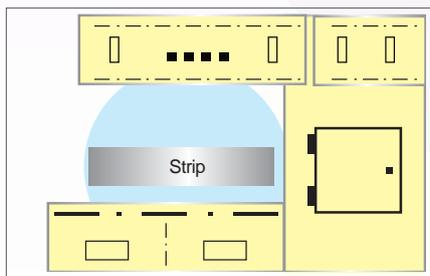
The thickness deviation with the whole coil is automatically inspected by the X-ray generated system to assure the thickness accuracy.
