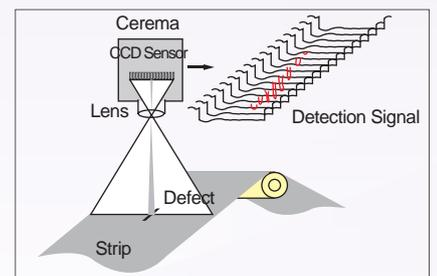
Both sides of strip surface with entire coil length are automatically inspected by the high resolution camera system to assure the strip surface quality.
