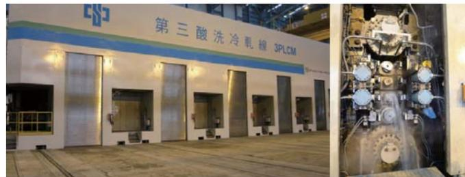
The pickled coils are rolled into specified thickness by cold rolled mills with controlled rolling force and strip tension. Based on strip center and edge part measurements of the thickness at the entry and delivery sides of the mills, either the strip center or edge thickness deviation is minimized by the computer-controlled system.
