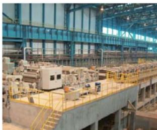
The main purpose of this stage is to remove the scale of hot rolled coil by heated solution of hydrochloric acid for its smooth surface finish.
