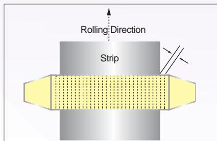
The rolling controlled could be dynamically adjusted depending on the simultaneous measurement result of strip flatness by shape-meter roll.
