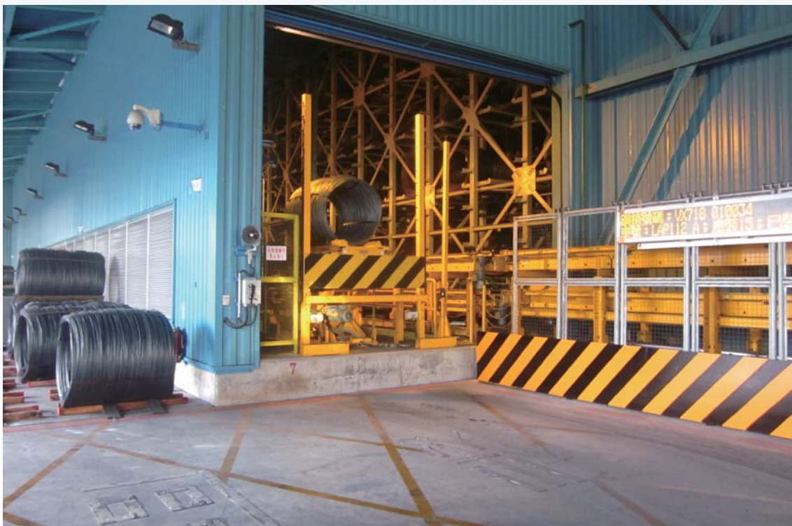
2. The coils after rolling can be moved into the system automatically, which the appearance of the coils keeps quality well.
