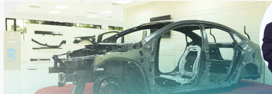
▲ "Interstitial Free Automobile Steel containing 30% Recycled Content" is ideally suited for processing into complex interior and exterior automotive body panels.
