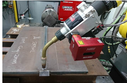
Fig.5. Lincoln S-500, combined with a Fanuc M20iA robot, performs welding in the laboratory.
