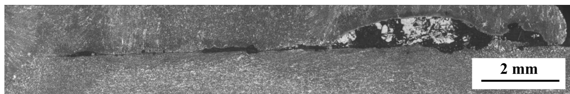
Fig.7. Micro-metallographic of the poor fusion zone indicated in the yellow box area in figure 6.
