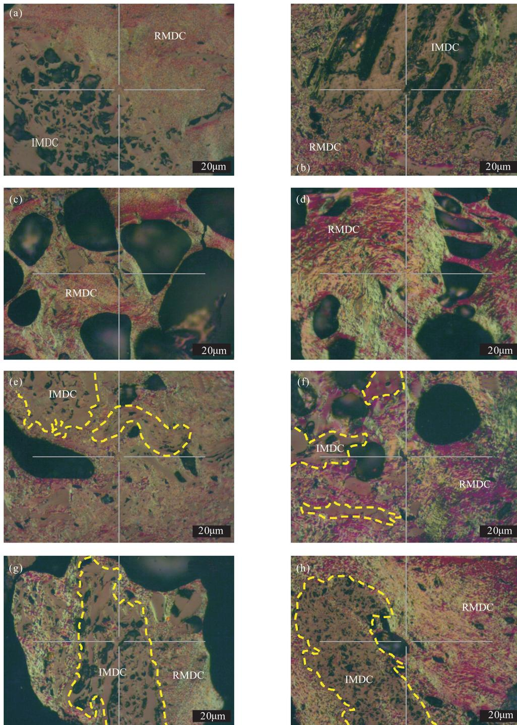
**Fig.6.** Polarized reflected light microscope images (a) AU-1 (b) AU-3 (c) IN-2 (d) IN-5 (e) AM-1 (f) AM-2 (g) AF-1 and (h) AF-2.
