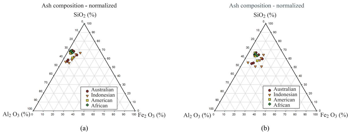
**Fig.3.** Ash composition results of metallurgical coals from different regions. (a) Comparison with  $Fe_2O_3$ , (b) Comparison with Alkali (Alkali (%) =  $K_2O$ (%) +  $Na_2O$ (%) +  $MgO$ (%) +  $CaO$ (%) +  $Fe_2O_3$ (%)).
