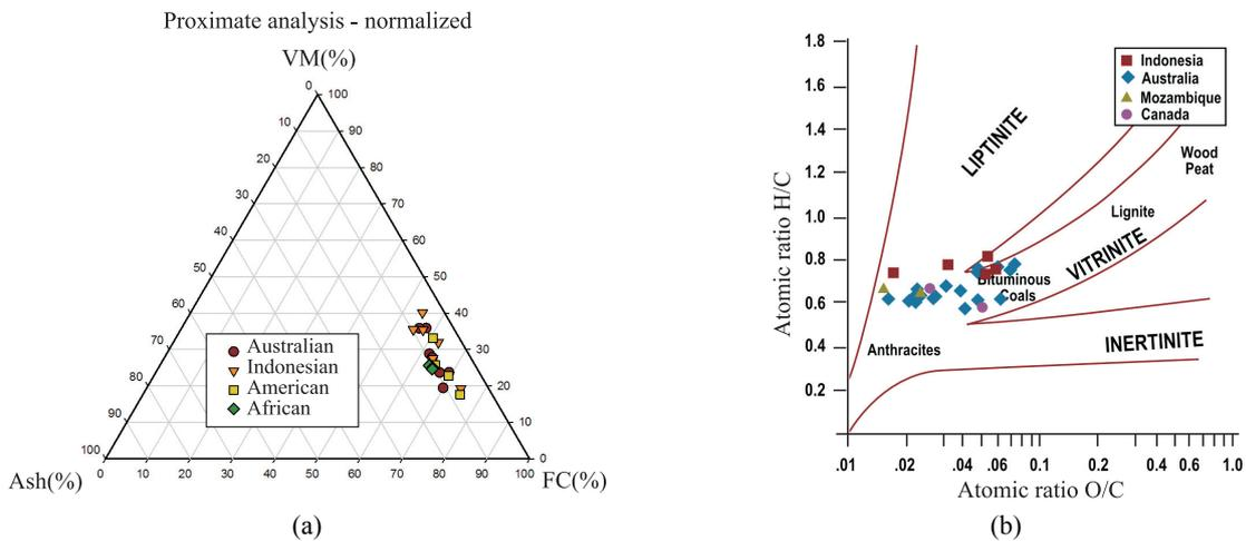
**Fig.2.** Proximate and Ultimate analytic results of metallurgical coals from different regions. (a) Proximate analysis results shown in ternary plot (b) Ultimate analysis results shown in the atom ratio plot.
