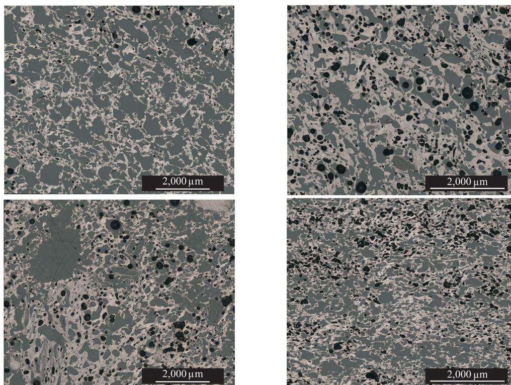
**Fig.7.** Large scale microscope images of cokes from Indonesian coals (a) IN-4 (b) IN-3 (c) IN-5 and (d) IN-6.
