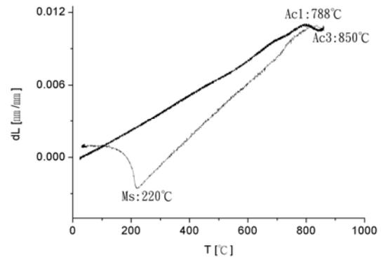
**Fig. 4.** Phase transformation point of the newly developed steel examined by dilatometer.
