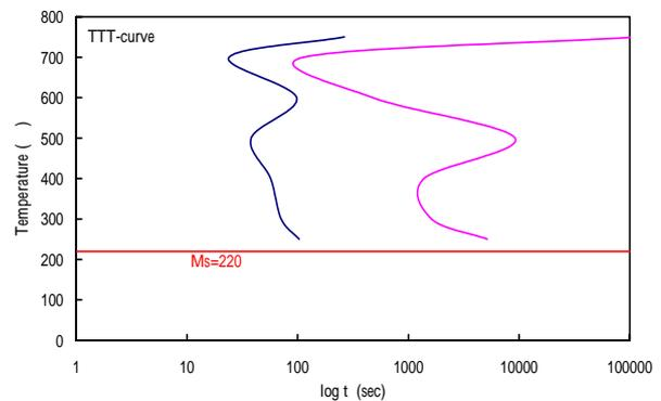
**Fig. 5.** TTT diagram for the newly developed steel.
