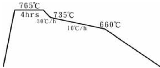
Fig. 1. Spherical annealing patent for the newly developed steel.
