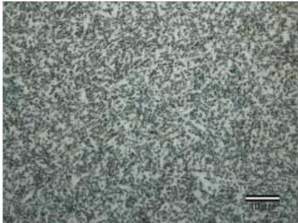
Fig. 2. Spherical annealing microstructure for the newly developed steel.
