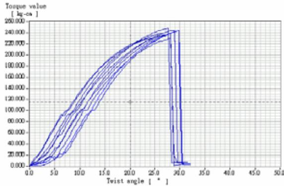
Fig. 12. Torsion curve by torsion test for the newly developed steel
