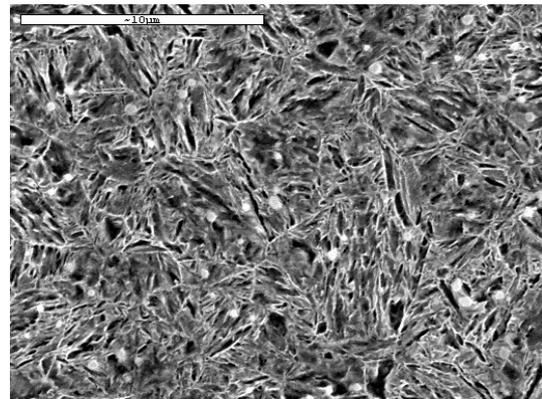
**Fig. 11.** SEM morphology for oil quenching (860 °C -15min.) and tempering (170 °C -2hrs) specimen.
