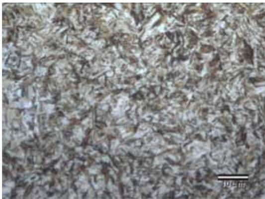
**Fig. 8.** OM morphology for 860 °C -15min. austenitizing and oil quenching specimen.
