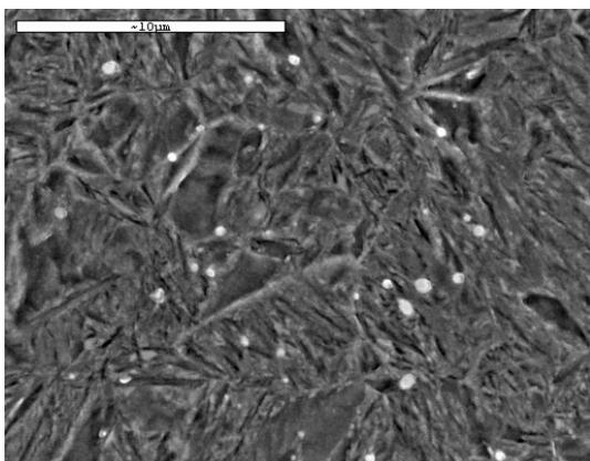
**Fig. 9.** SEM morphology for 860 °C -15min. austenitizing and oil quenching specimen.
