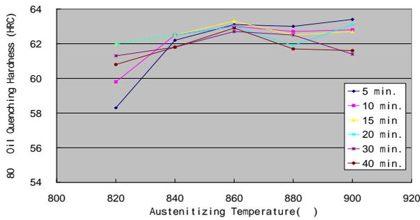
**Fig. 7.** Hardness curves of oil quenching specimens for the newly developed steel.
