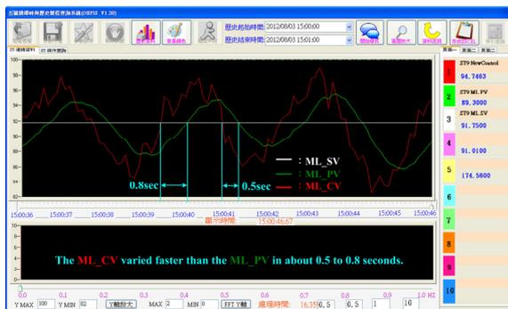
Fig.7. Effect of the sliding mode controller in the MLC circuit.
