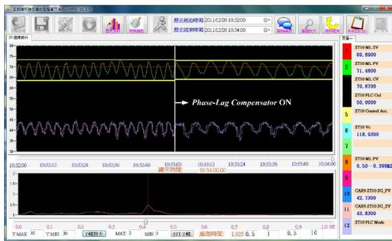
Fig.6. Phase-lag compensator testing result.
