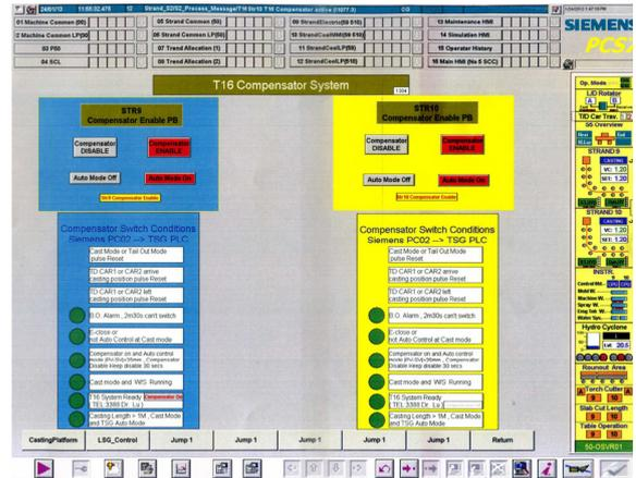
Fig.4. HMI of the software switch.
