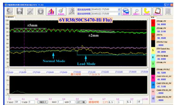
Fig.5. Phase-lead compensator testing result.
