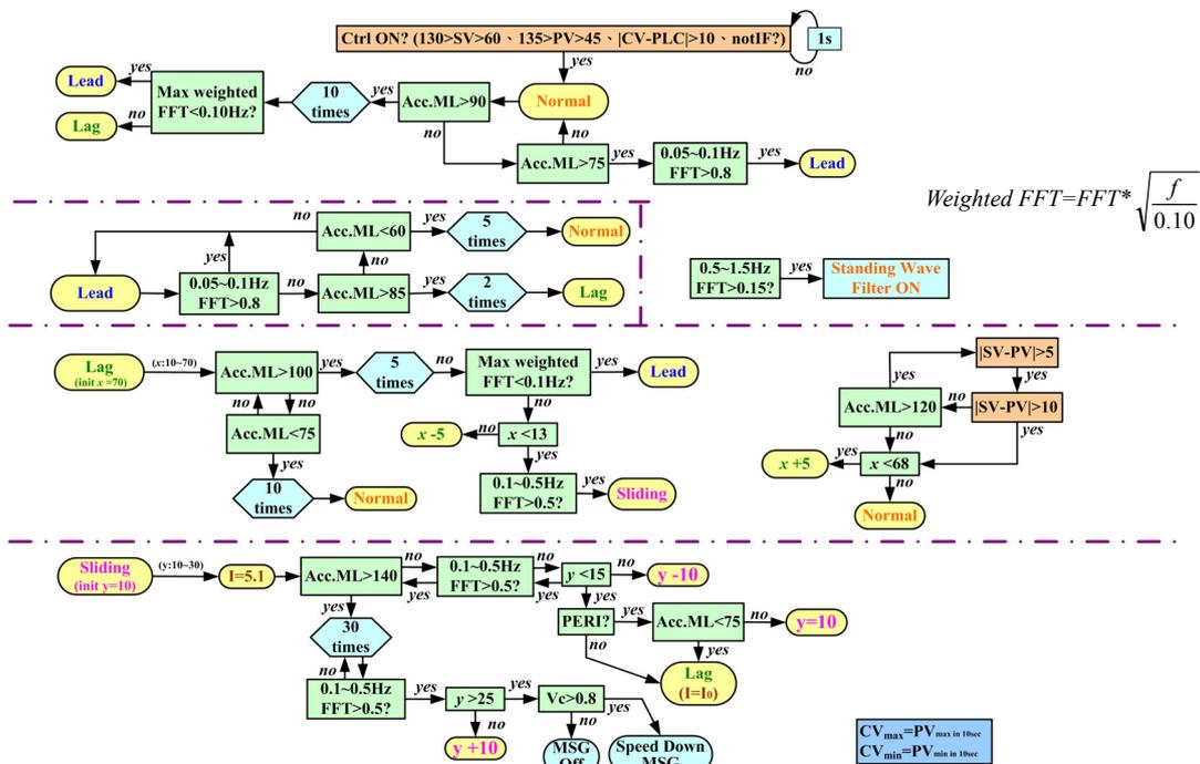
Fig.2. MLC compensator decision logic.
