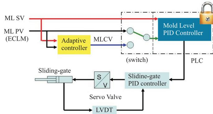
Fig.1. Adaptive mold level control diagram.
