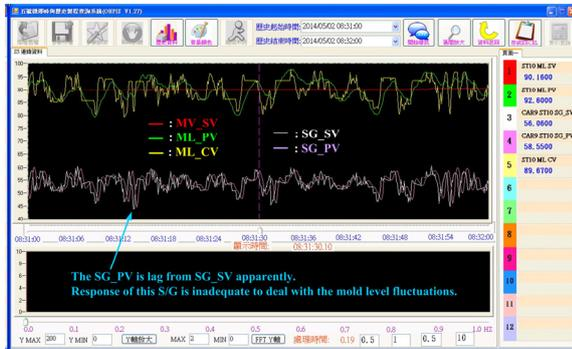
Fig.10. Response of the sliding gate at CSC #5 slab C.C.
