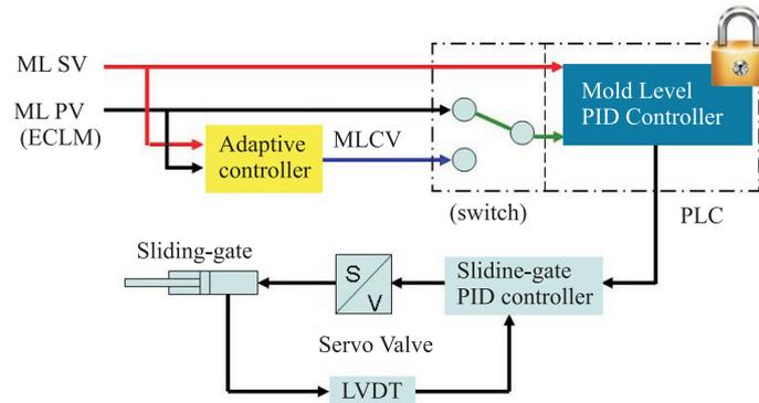
Fig.1. Adaptive mold level control diagram.
