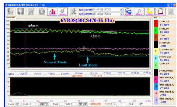
Fig.5. Phase-lead compensator testing result.
