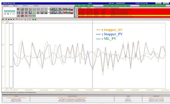
Fig.11. Response of the stopper at DSC #2 slab C.C.
