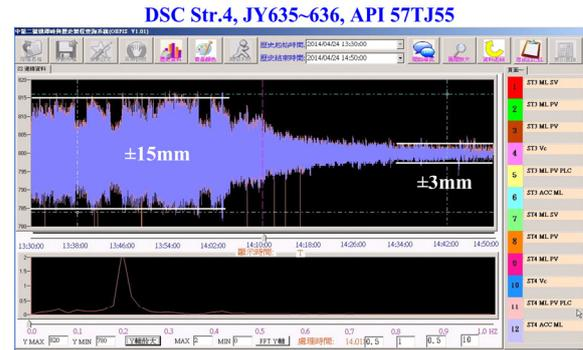
Fig.8. Sliding mode controller testing result.
