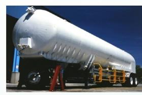
Tank truck was made of pressure vessel steel.
