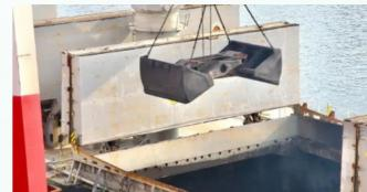
Unloading grab at CSC Group terminal was made from CSC's abrasion resistant steel plates.
