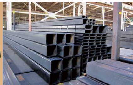
Structural square tube
