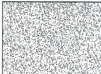
Rust Grade 3-P, 16% Rusted
