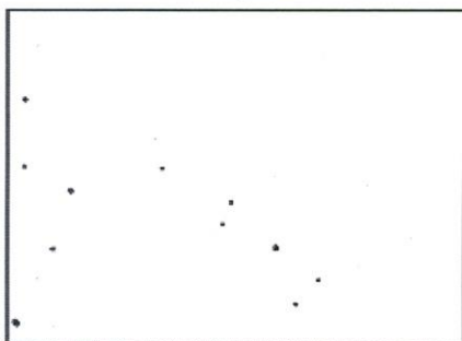
Rust Grade 8-P, 0.1% Rusted
