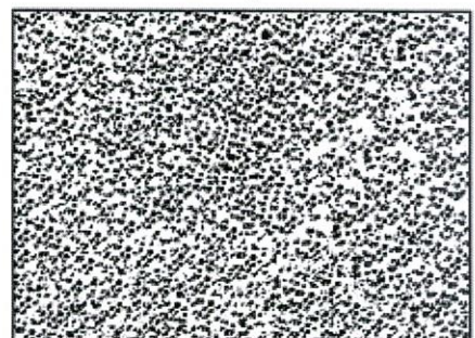
Rust Grade 2-P, 33% Rusted
