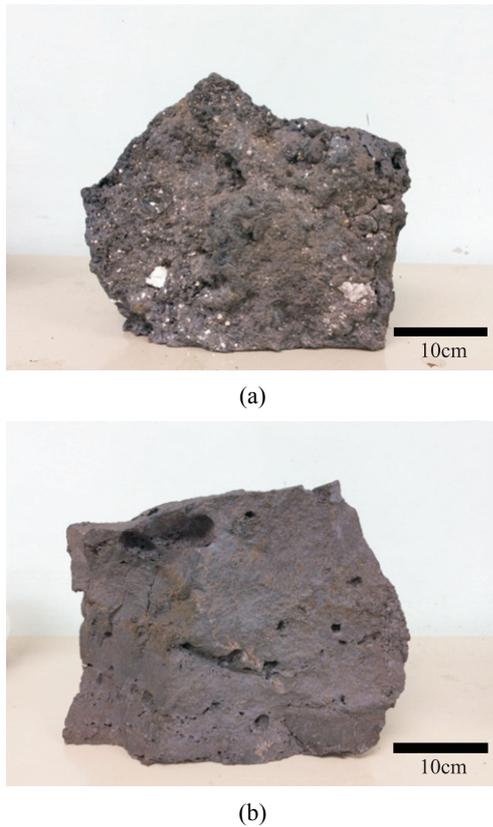
**Fig.4.** The pictures of the BOF slag (a) without HBM and (b) with HBM treatment.
