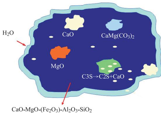
**Scheme 1.** The compositional inhomogeneity of BOF slag shows minerals (e.g. f-CaO/MgO, dolomite and C3S) are included in the slag. Only f-CaO/MgO that is exposed on the surface of slag can be hydrated by water and stabilized. Therefore, hydration-based methods are not practical for stabilizing BOF slag.
