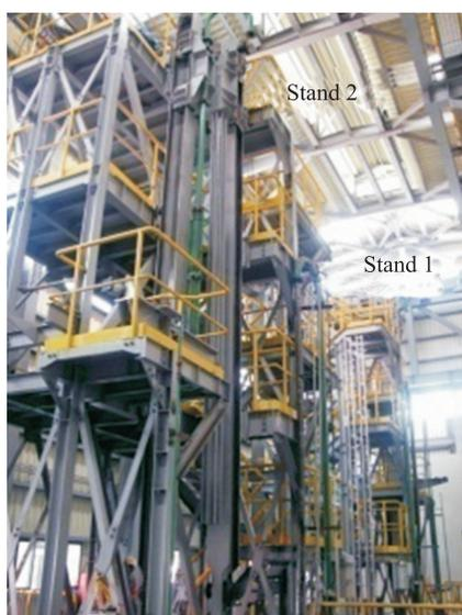
**Fig.1.** The HBM setup consists of 2 stands and both of them can be operated independently to execute slag modification.
