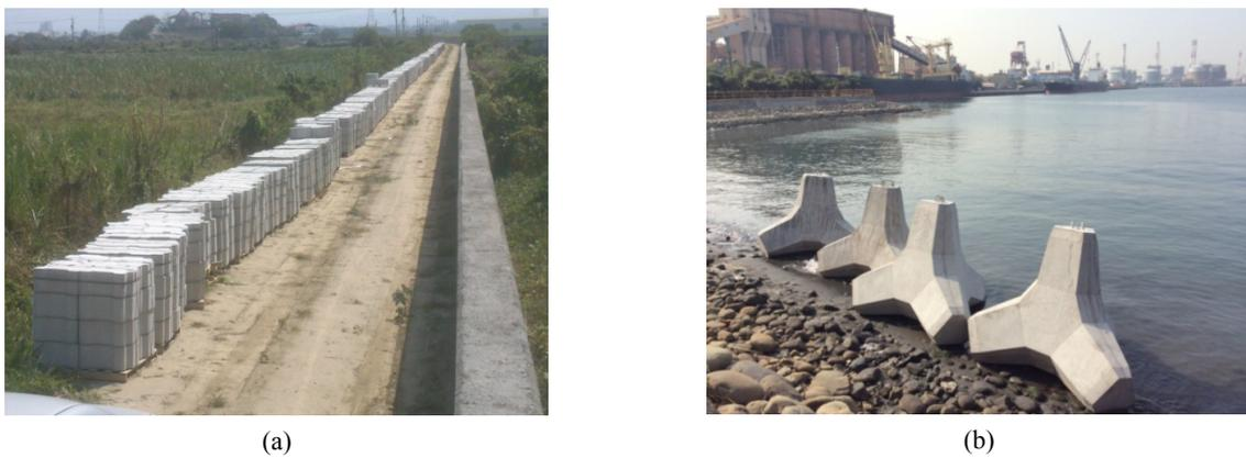
**Fig.7.** (a) The revetment blocks (size: 50×50×25 cm<sup>3</sup>) and (b) Tetrapods (10 t/unit) made of 40 wt.% of modified BOF slag are now placed outdoors for field tests.
