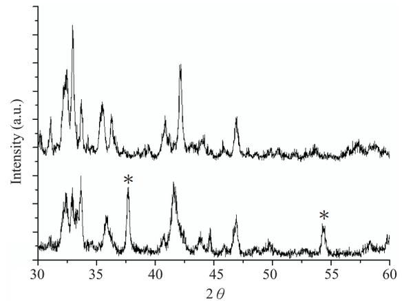
**Fig.5.** The XRD pattern profiles of BOF (bottom) and modified BOF slag (top), respectively. The stars denote the phase of f-CaO.
