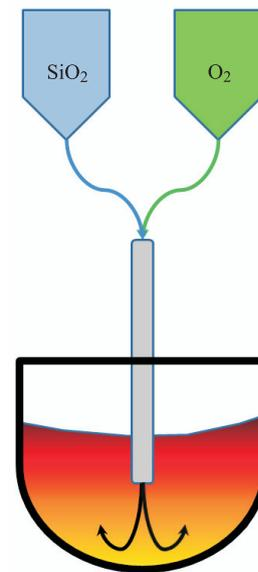
**Scheme 2.** The concept of the HBM technique. By blowing oxygen into the molten slag, this oxidation reaction of FeO occurs, which generates heat for maintaining the temperature of molten slag.
