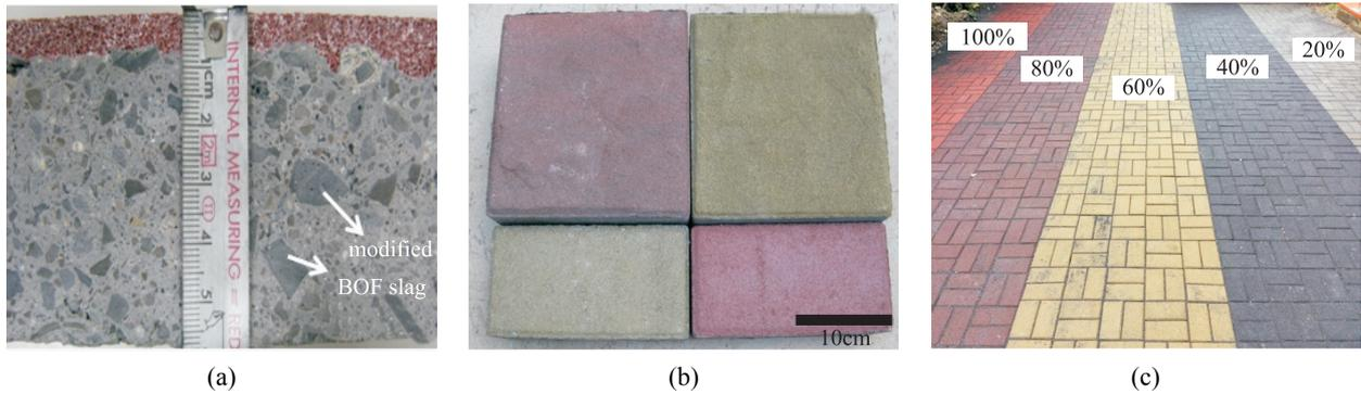
**Fig.6.** (a) The modified BOF slag is utilized as a raw material for making bricks, (b) The pavement/grass bricks with a variety of colors and sizes can be made by using modified BOF slag as a raw material, (c) Pavement bricks with different levels of modified BOF slag substitute paved outdoors demonstrate good volumetric stability.
