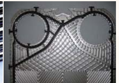
The heat-exchanger equipment produced by pure Titanium cold-rolled coil.
