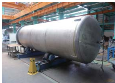
The chemical storage tank produced by pure Titanium heavy plate.
