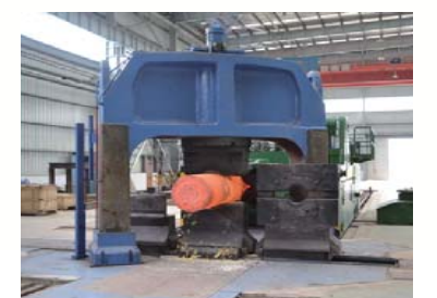
1600 Tons Forging Facility
