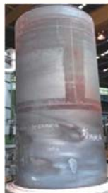
Inner chamber material application for high temperature furnace by using Alloy 800H plate
