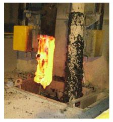
**Fig.2.** Each stand of the HBM setup is equipped with a lance (right) for injecting additives, a rod (left) for breaking solidified slag, and collecting samples. The rod covered by molten slag after collecting samples is displayed.
