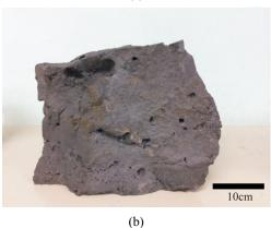
**Fig.4.** The pictures of the BOF slag (a) without HBM and (b) with HBM treatment.
