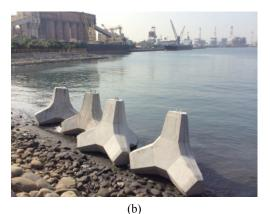
**Fig.7.** (a) The revetment blocks (size:  $50 \times 50 \times 25$  cm<sup>3</sup>) and (b) Tetrapods (10 t/unit) made of 40 wt.% of modified BOF slag are now placed outdoors for field tests.
