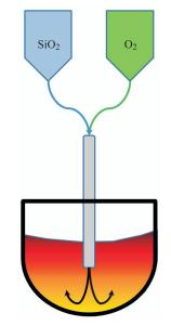
*Scheme 2.* The concept of the HBM technique. By blowing oxygen into the molten slag, this oxidation reaction of FeO occurs, which generates heat for maintaining the temperature of molten slag.
