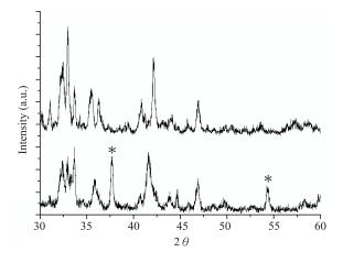
**Fig.5.** The XRD pattern profiles of BOF (bottom) and modified BOF slag (top), respectively. The stars denote the phase of f-CaO.
