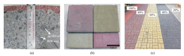
**Fig.6.** (a) The modified BOF slag is utilized as a raw material for making bricks, (b) The pavement/grass bricks with a variety of colors and sizes can be made by using modified BOF slag as a raw material, (c) Pavement bricks with different levels of modified BOF slag substitute paved outdoors demonstrate good volumetric stability.
