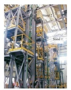
**Fig.1.** The HBM setup consists of 2 stands and both of them can be operated independently to execute slag modification.
