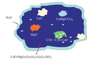
**Scheme 1.** The compositional inhomogeneity of BOF slag shows minerals (e.g. f-CaO/MgO, dolomite and C3S) are included in the slag. Only f-CaO/MgO that is exposed on the surface of slag can be hydrated by water and stabilized. Therefore, hydration-based methods are not practical for stabilizing BOF slag.
