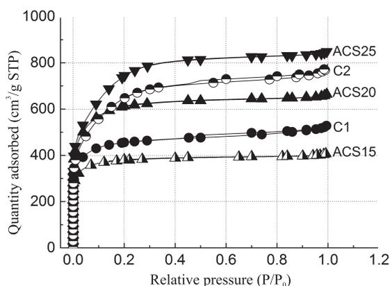
**Fig.1.** The isotherms of N<sub>2</sub> on activated of ACS-series and C-series activated carbons at 77 K.
