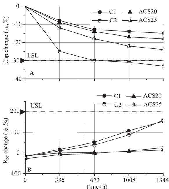
**Fig.3.** The aging performances of EDLCs of the electrode made of ACS-series and C-series activated carbons.
