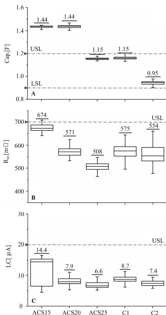
**Fig.2.** The initial capacitance (A), DC resistance (B) and leakage current (C) of EDLC of the electrode materials made of ACS-series and C-series activated carbons.
