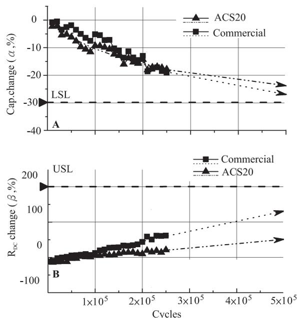
**Fig.4.** The cyclic charge-discharge performances of EDLC of the electrode made of activated carbon ACS20, and those of a commercial EDLC.
