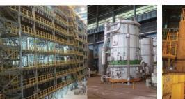
The steel strip is significantly hard and brittle after cold rolling which the grains are elongated along with lots strain energy. To obtain the desired mechanical properties of strip, the coils shall be piled and covered by the box which called batch annealing or the strip is continuous treated in furnace which called continuous annealing. Both annealing technology are possessed in CSC according to different product requirements.
