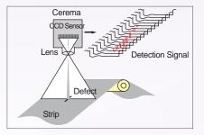
Both sides of strip surface with entire coil length are automatically inspected by the high resolution camera system to assure the strip surface quality.
