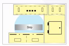
The thickness deviation with the whole coil is automatically inspected by the X-ray generated system to assure the thickness accuracy.
