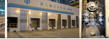
The pickled coils are rolled into specified thickness by cold rolled mills with controlled rolling force and strip tension. Based on strip center and edge part measurements of the thickness at the entry and delivery sides of the mills, either the strip center or edge thickness deviation is minimized by the computer-controlled system.
