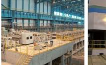
The main purpose of this stage is to remove the scale of hot rolled coil by heated solution of hydrochloric acid for its smooth surface finish.
