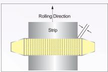
The rolling controlled could be dynamically adjusted depending on the simultaneous measurement result of strip flatness by shape-meter roll.
